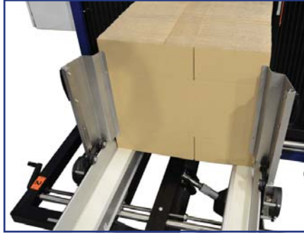
Blank Delivery Control Powered belts precisely govern the delivery speed of the case blanks. Blank retainers ensure the blanks are spaced correctly.
